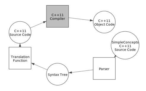
Fig. 5. The SimpleConcepts approach. Circles indicate input and output artifacts, and rectangles indicate processes. Pre-existing components are colored gray.
